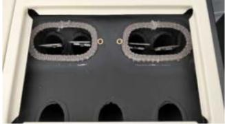
The left cleaning levers are used to clean the left part of the vertical heat exchanger while the right cleaning levers are used to clean the right part of the exchanger.
